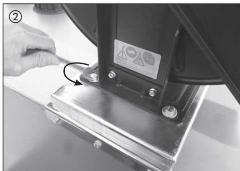
② Install hose reel on console with: 4 x hex bolts M 8x16 4 x washers A 8.4
